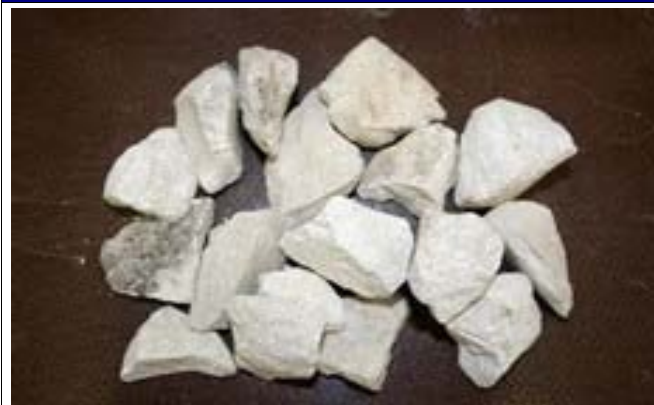
Lime after 3 hours at 1050°C
